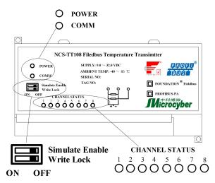
Figure 4.4 DIP switch of NCS-TT108 Smart Temperature Transmitter
