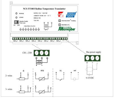
Figure 2.6 Temperature transmitter connection
