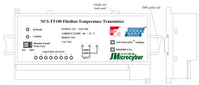
Figure 2.1 Mount of guide rail
