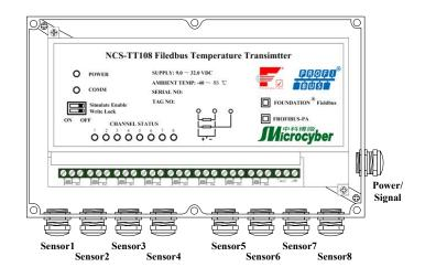
Figure2.7 Cable sealing connector
