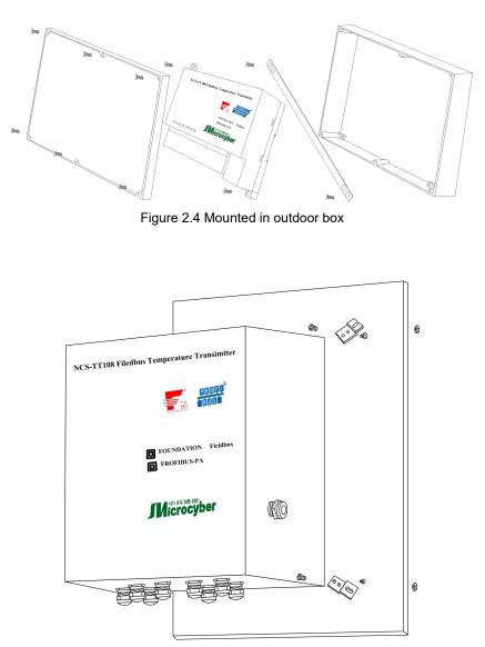
Figure 2.5 Outdoor case surface mounting
